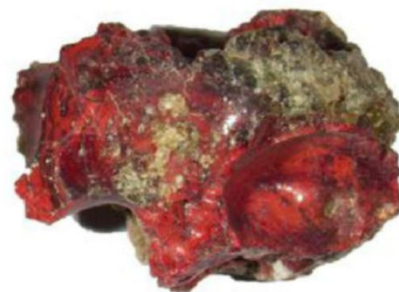
A new clathrate was found in this trinitite sample from the Manhattan Project's bomb blast.
