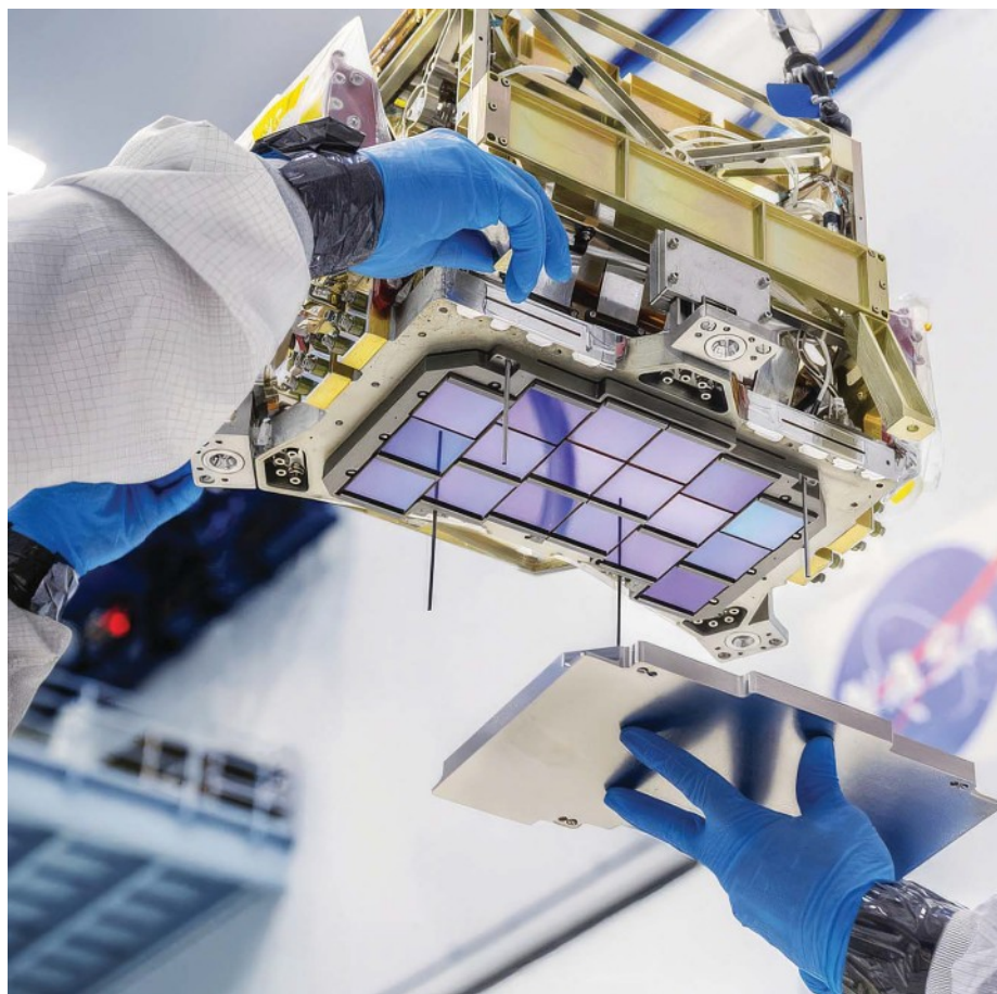
Technician Billy Keim prepares to install the protective cover over the 18 detectors of Roman’s Wide Field Instrument at NASA’s Goddard Space Flight Center in Greenbelt, Maryland. NASA/CHRIS GUNN
